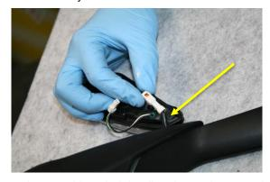
9. Insert cable, mind the direction and connect indicators
