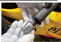
Remove the bar ends with the appropriate tools needed.
