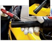
Check the (right side) throttle tube for any ridges. If there are any, they must be removed using a dremel tool.
