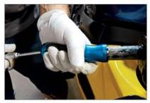
Using an air compressor and hose, install the grip while using the air to expand and move the grip onto the bar.
