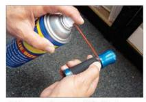
4. Place a small amount of WD-40 between the D3 rings and the krayton gel grip. Clean the left and right side of any dirt or old glue.
