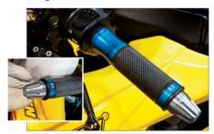
6. After both grips have been successfully installed, re-install your bar ends. Let grips sit for at least 1 hour in order for the WD-40 to evaporate. You are finished.
