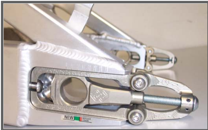
View: KTS-SP1-* guidance part with slider and adjusting bolt
